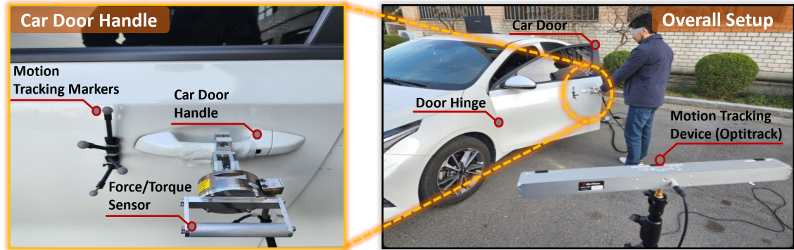
Figure 5.2: Experimental setup for recording car door force profiles and angular motion. A force sensor was attached to the door handle, and OptiTrack markers were placed to track the door's position during opening.
